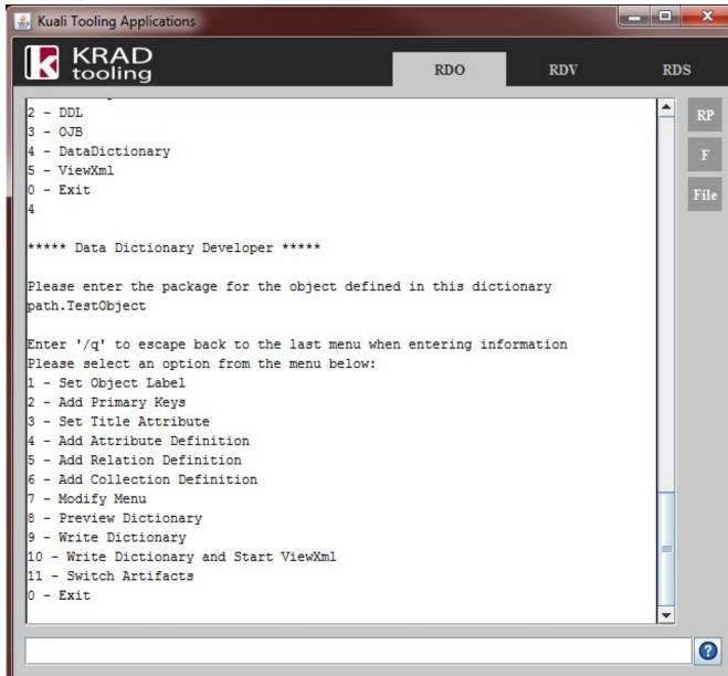
The Data Dictionary File is a xml file generated using the Spring Beans format. The Dictionary contains information on the a single Data Object. This includes ways to identify it and its different properties. It also contains definitions for each property to aid in the validation of information it holds.
