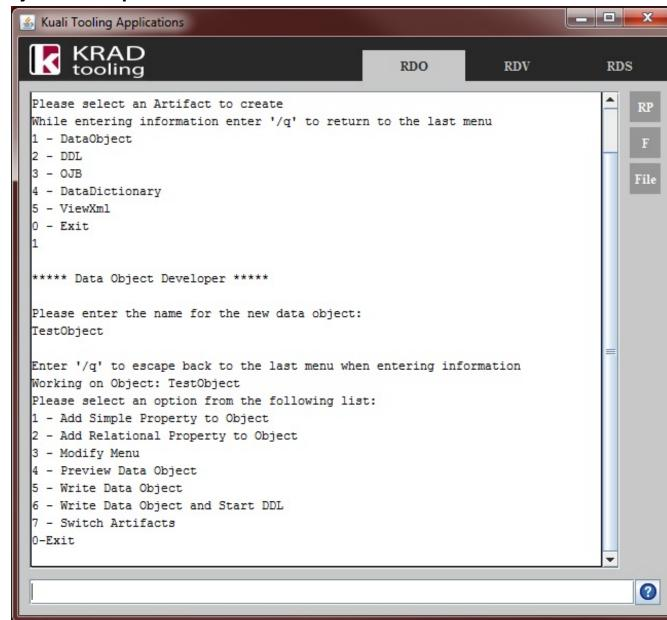
The Data Object is a simple java class that contains a number of properties (data entries). These properties can consist of simple data types like int, String or boolean, or relation (user defined) data types. For each data type the needed imports, declarations and constructor initializion is created, as well as the getters and setters needed to fill or retrieve that data stored for these properties.
